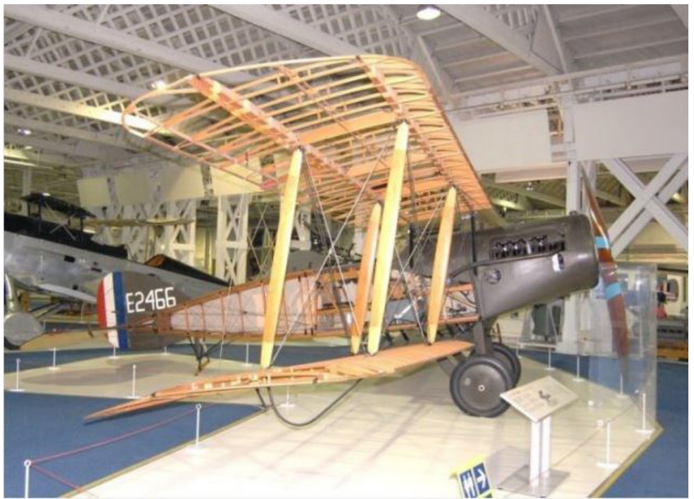
Bristol Fighter restored using one of the airframes
